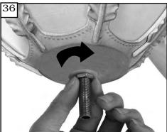
Install cage with glass onto light kit, install rubber washer and hex nut to hold in place and tighten in direction of arrow.
